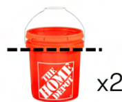
Figure 22. A bushel is typically measured in the field using a 5 gallon bucket with a designated 4 gallon fill line twice to measure a total of 8 gallons.
