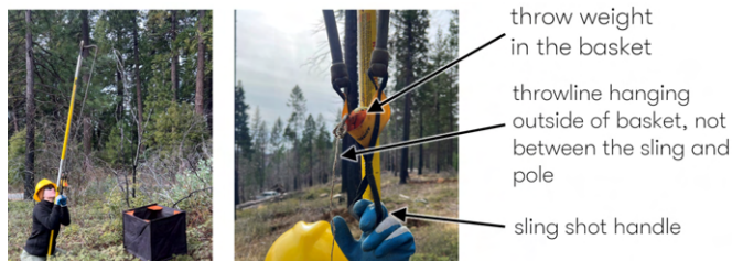
Figure 4. Set up for Big Shot Sling Shot aim, weight, and throwline.
