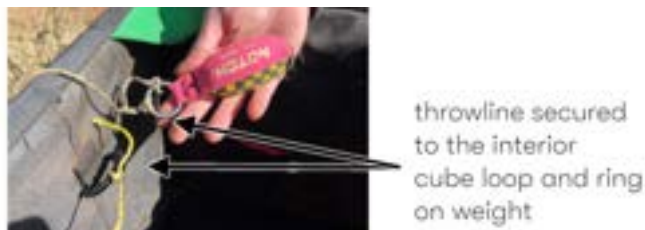
Figure 2. Throwline secured to cube and weight.
