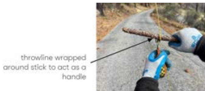
Figure 6. Throwline wrapped around stick to create handle for pulling on line.
