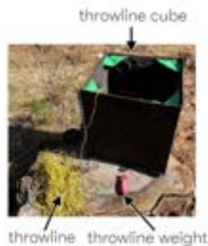
Figure 1. Throwline kit with cube, line, and weight.
