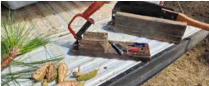
Figure 24. Cone cut tests of ponderosa pine using cone cutters.
